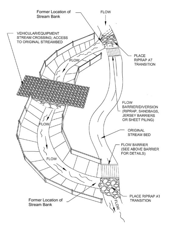
Figure TDM-1. Typical Temporary Diversion Channel
